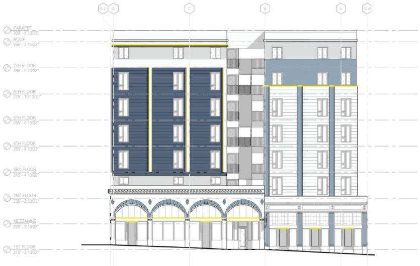
2 EXTERIOR LIGHTING ELEVATION - BANCROFT 3/32" = 1'-0"
